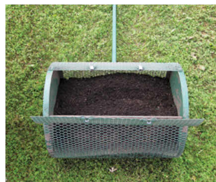
Figure 5b. Manual compost spreader. ( Lloyd Jensen )
